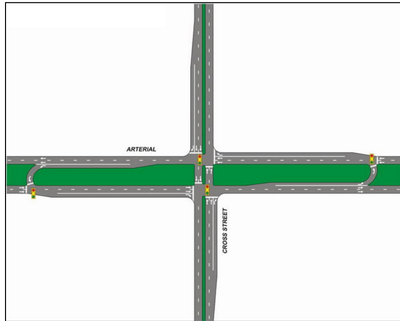
Figure 1 Typical median U-turn intersection (UMD, 2004)
